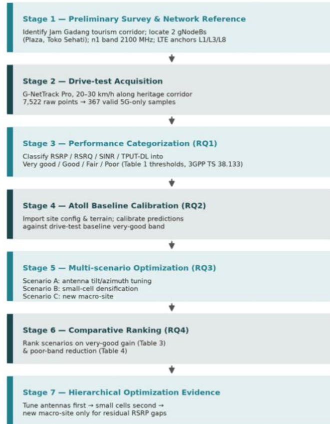
Fig. 1 Research workflow: drive-test acquisition, spatial filtering, Atoll baseline calibration, multi-scenario optimization, comparative ranking, and the resulting hierarchical optimization evidence.
