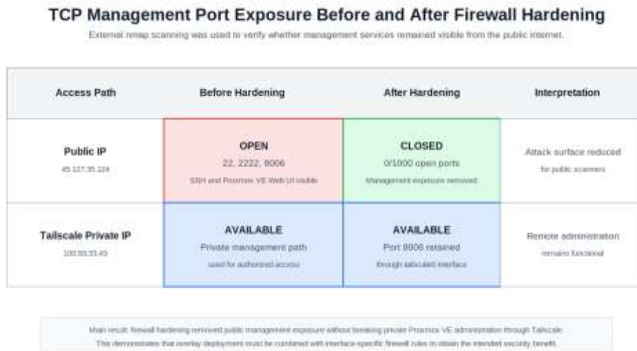
Figure 6. TCP management port exposure before and after firewall hardening
