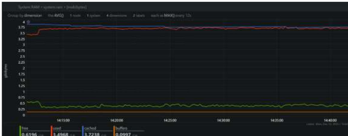
Fig. 4 System memory utilization during sequential pipeline execution using Local Orchestrator under light workload
