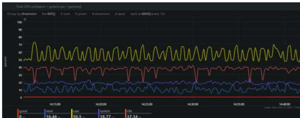
Fig. 3 CPU utilization profile during sequential pipeline execution using Local Orchestrator under light workload
