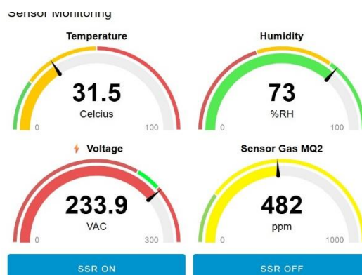
Gambar 2 Tampilan Dashboard Monitoring Lokal LoRa Smart Home
